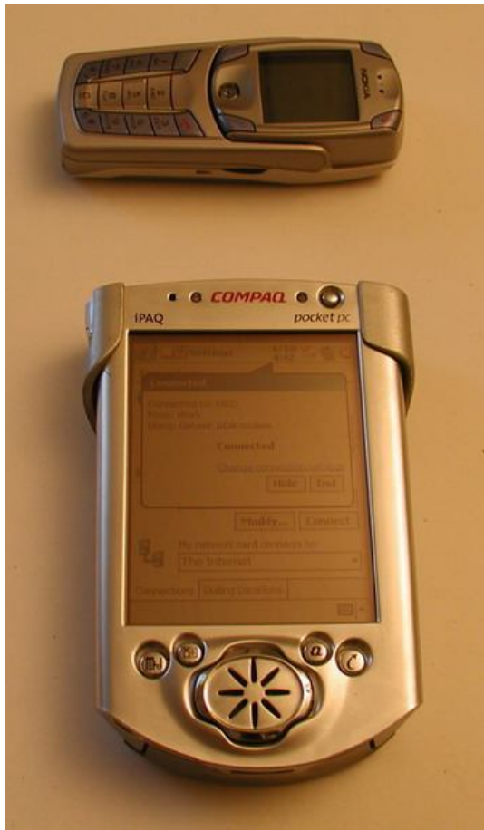
iPAQ 3650 connected to the Nokia 6820 over IR to the net over GPRS/EDGE. The next PDA will be connected over Bluetooth
